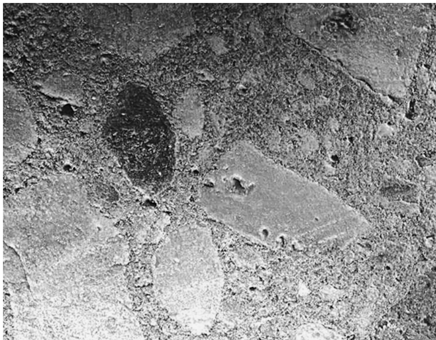
Figure 3 Pit formation in cement matrix and aggregate. Concrete 55; location: zone II (4 mm away from zone I); image width: 17 mm; t_E = 5 s.
